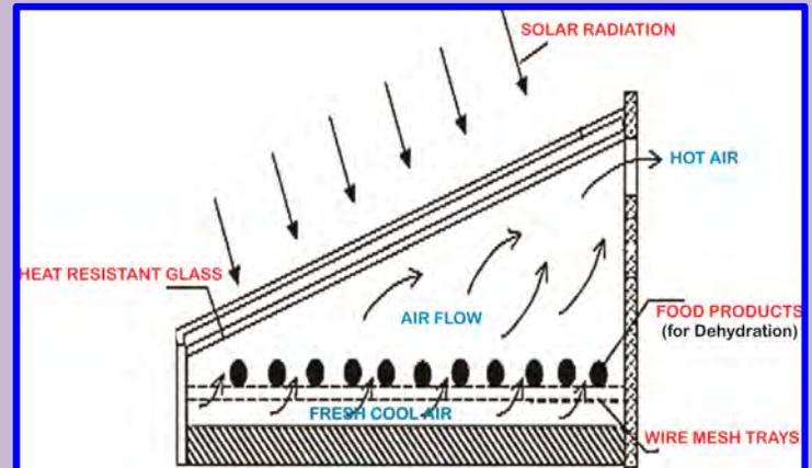
Dehydration Process in Mini Solar Dehydrator
